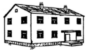
DG 1: Slight Damage
