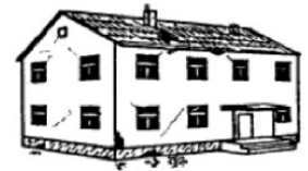
DG 2: Moderate Damage
